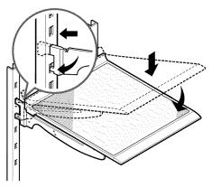
**A CAUTION:** Make sure that shelves are level from one side to the other. Failure to do so may result in the shelf falling or spilling food.
